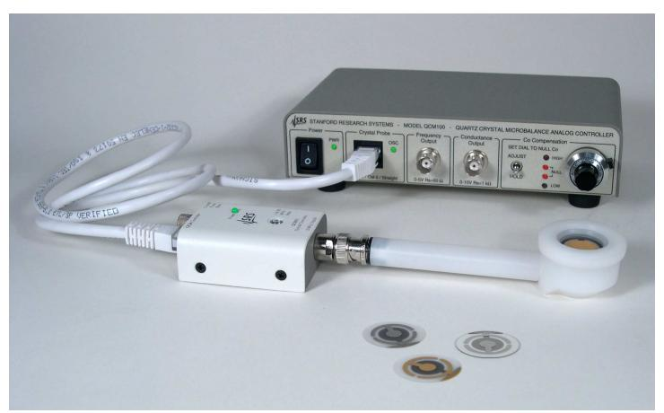
quartz crystal resonator with the necessary gain to overcome viscoelastic losses and achieve series resonance, while providing a signal that monitors the energy dissipated by the sensor (i.e. related to the series resonance resistance). The crystal oscillator will reliably drive crystals with resistance up to 5 k $\Omega$ . For example, it will maintain oscillation in viscous aqueous solutions containing over 88 % glycerol (w/w %).
